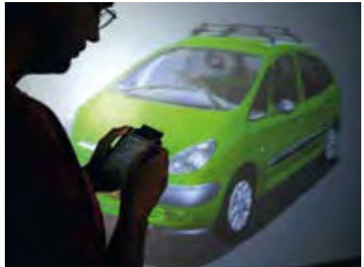
ARSBOX (2001) virtual prototyping using a PALMIST, which allowed users not only to change static parameters but also to control the dynamics of a VR-world.
