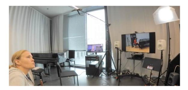
At first, the camera and the screen in Malmö were placed on the left side. This initially caused some complications until it was moved more into the middle, straight in front of the Malmö duo. It was also noted that the height of the camera highly affected the performing area for the singers. The LoLa camera in Malmö was placed lower than in the Sibelius studio, where it's placed in the ceiling. Therefore, Therefore, Wilén had to adjust her area of movement in order not to go out of the picture.
